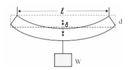
A bar of length I, breadth b, and depth d when loaded at the centre by a load W sags by an amount given by  $\delta = W I^3/(4bd^3Y)$
